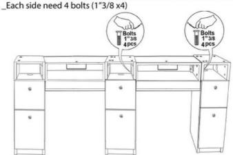
Install Bolts from the inner side flap of the two side cabinet tables \_Each side fit 4 bolts (1"3/8 x4)
