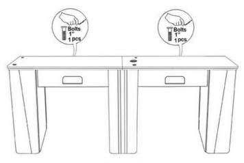
Install Bolts from the innerside of the marble table onto the marble top \_Each side fit 1 bolt (1"1/4 x2)
