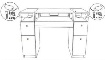
Install Bolts from the inner side flap of the two side drawer tables
