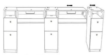
Step 4: Installing right drawer tables \_Install right side face table first then side table with cabinets after.
